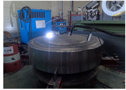
GTAW WELDING (DISC)
